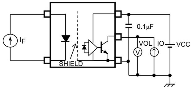
**TEST CIRCUIT 3:  $I_{CCL}$  Test Circuit**
