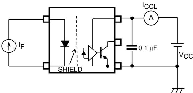
**TEST CIRCUIT 4:  $I_{CCH}$  Test Circuit**
