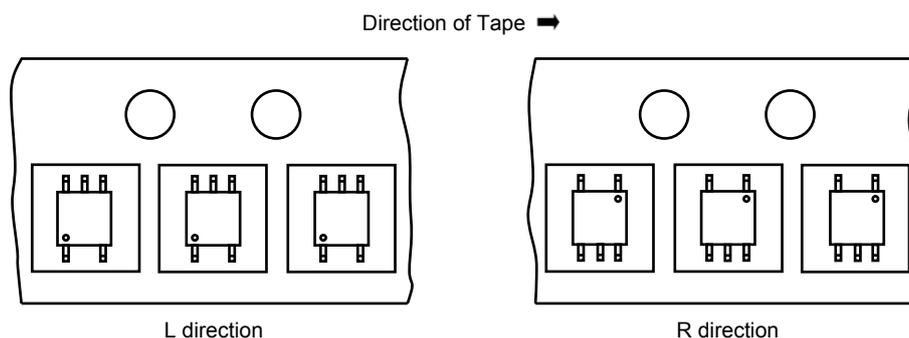
Figure 1 Device Orientation
