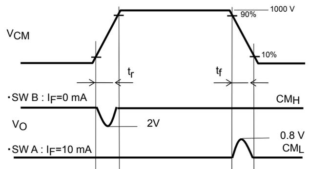
$$CM_H = \frac{800(V)}{t_r(\mu s)} \quad CM_L = \frac{800(V)}{t_f(\mu s)}$$
